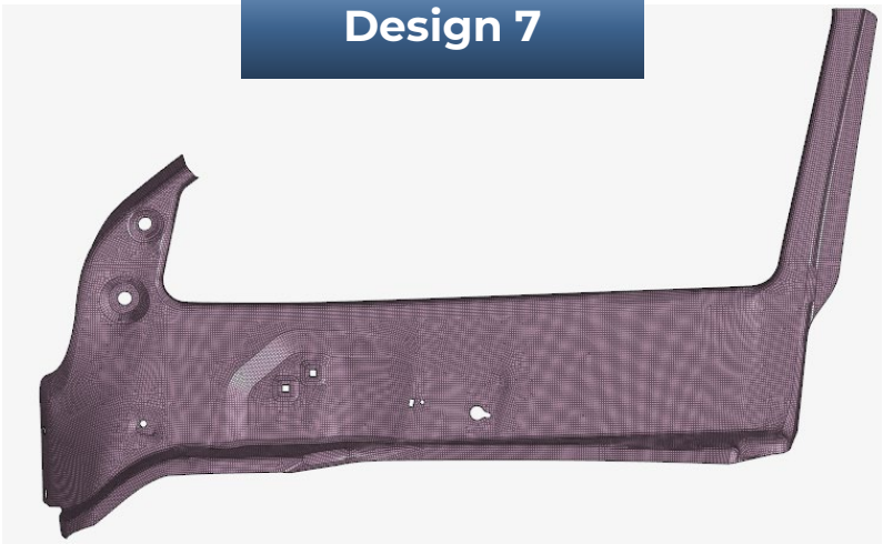
2-Layer 100% Dense (Alternating) Glass and Carbon
