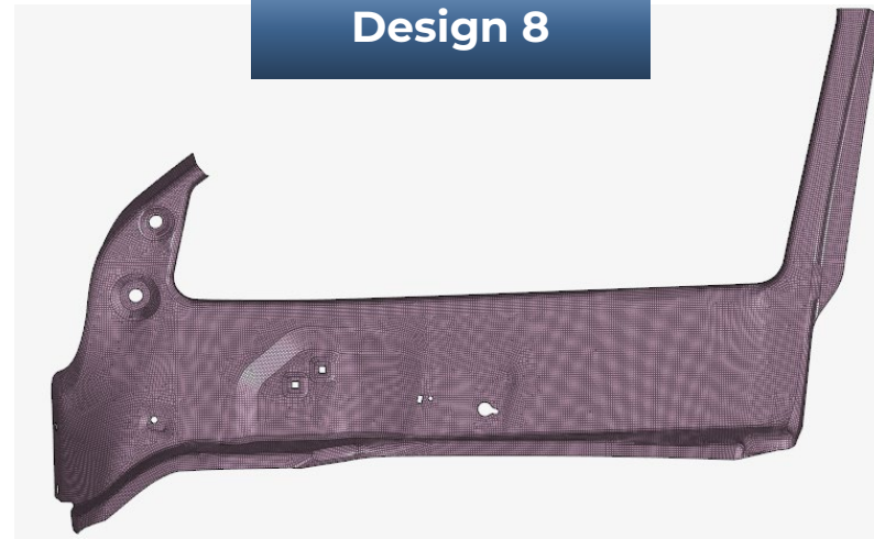
2-Layer 100% Dense Carbon Inner, Glass Outer
